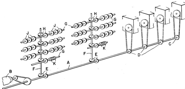
The Harvard Mark I [17, 21, 2, 45, 26, 3, 29] was a relay computer that took instructions from a paper tape and used the position of wheels to store numbers. During transfers or additions, pulses operated clutches that momentarily linked the wheels to continuously turning drive shafts. When advancing from nine to zero, a cam operated a relay that tracked the presence of an outstanding carry.
