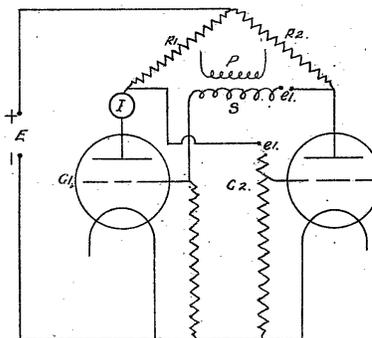
ring counter, only one flip-flop in the ring is on at any given time, and each incoming pulse causes the current flip-flop to turn off and the next one to turn on.
