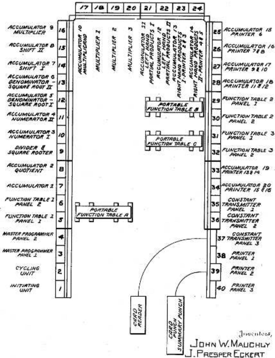
The ENIAC[17, 22, 21, 2, 45, 26, 3, 16, 6, 46, 44] was built for speed. It used about 18,000 vacuum tubes, cost over \$500,000 1946 dollars to build, consumed 174KW, occupied 1800 square feet, and weighed more than
