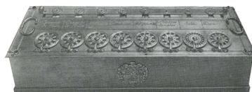
Blaise Pascal's Pascaline[40] could add numbers mechanically, including tracking carries between digits. Numbers were added by inserting a stylus into a hole in a wheel, and rotating the wheel.
