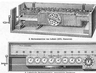
The Leibniz Calculator[41] could perform repeated addition, and addition at an adjustable digit offset, corresponding to multiplication by a power of ten. General multiplication could be achieved by repeating the
