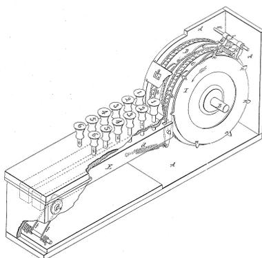
Key punch operated adding machines[23] allowed numbers to be added into a running total merely by pressing the appropriate keys. Mathematical functions could be looked up in a book of function tables, or computed using appropriate algorithms[1].
